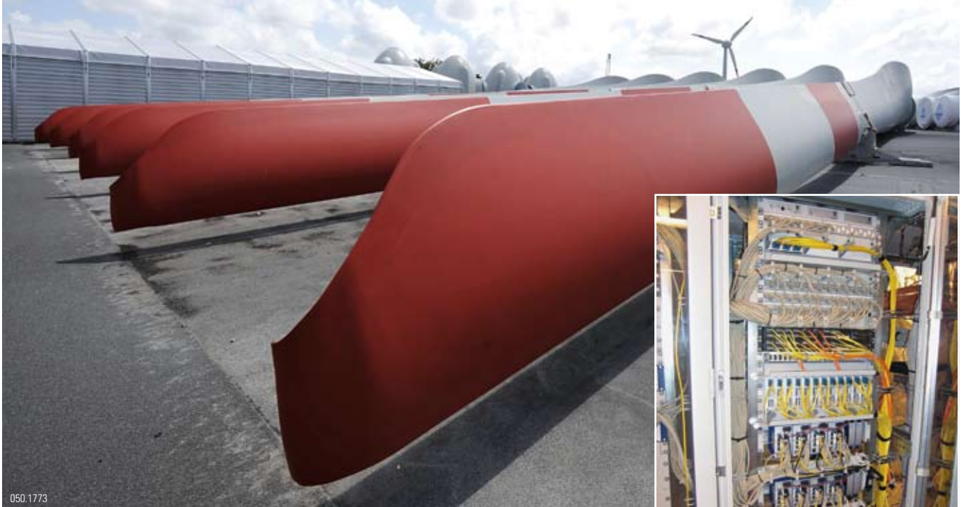
Offshore rotor blades in front of the factory at BARD Emden Energy GmbH & Co KG; Each blade is nearly 60 meters long and weighs about 28 tons. (Source: BARD-Group)
