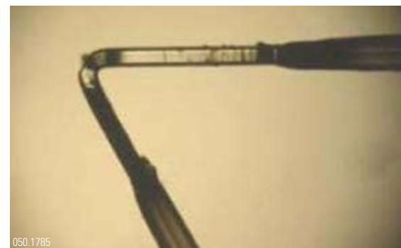
050.1785 If extremely high specific optical energy of 500kW/cm 2 (CATV networks) to MVV/cm 2 (transit networks with amplifiers) coincides with an extremely cramped space (no bending radii), then a) the transmission characteristics could be greatly disturbed and b) major fire damage could occur (examples are known from British Telecom, refer also to IEC 62547 TR Ed. 1.0).
