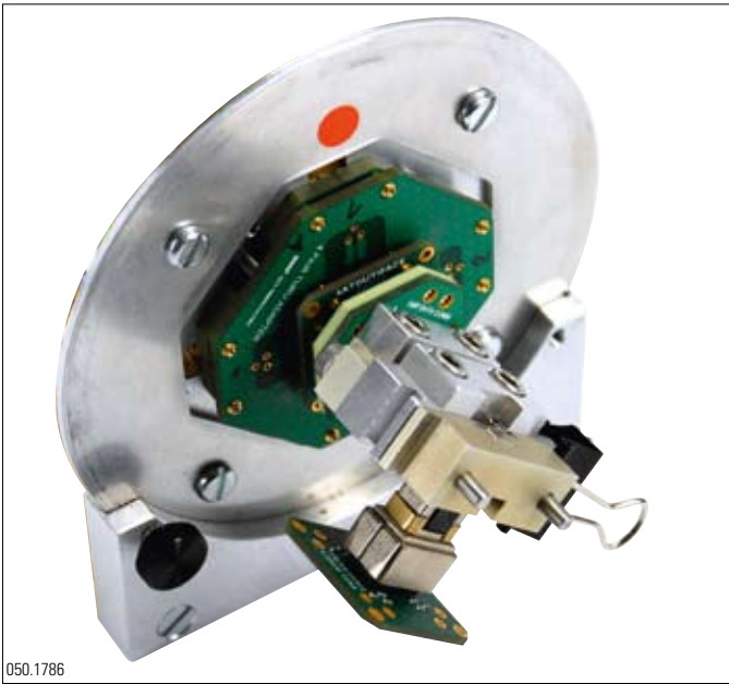
Reference plug on the direct probe fixture (DPF)
