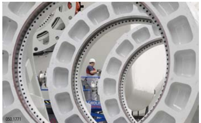
Machine holder in the assembly area for the BARD wind power plants in Emden: The cast-steel parts are about six meters in height and each weighs more than 70 tons. (Source: BARD-Group)
