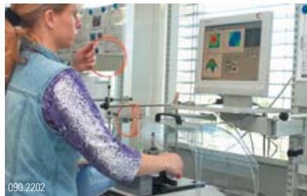
090.2202 Several inspection steps – such as the interferometry test – are necessary to achieve the high requirements.
