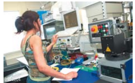
090.2204 Worst-case test: The attenuations measured at the factory are higher or the same in use as with a random connector pairing.
