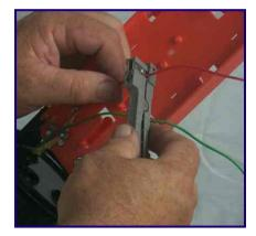
Carefully remove and clean the fibre tubes as not to damage the bare fibres.
