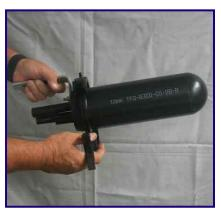
Open swing clamp and remove closure body.
