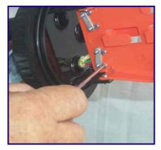
Position the open end of the cable A level with the entry port and tighten GRP link screws.
