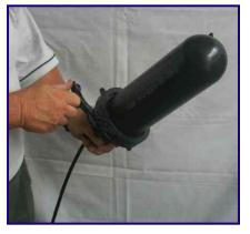
**23** Fit and tighten the swing clamp.
