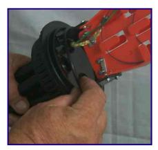
**21** Check that the O-ring is correctly seated and that the sealing surfaces on the base and body are clean and damage-free.
